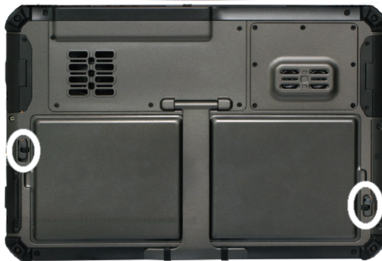
Figure 4: Battery latch locations on DT340T tablet
