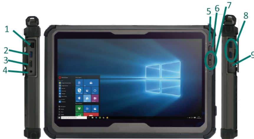
Figure 2: DT340T controls, indicators, and connectors
