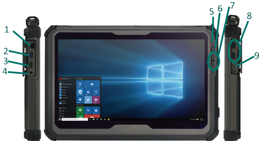
Figure 2: DT340T controls, indicators, and connectors
