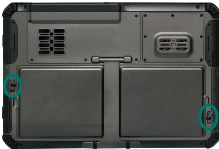
Figure 4: Battery latch locations on DT340T tablet
