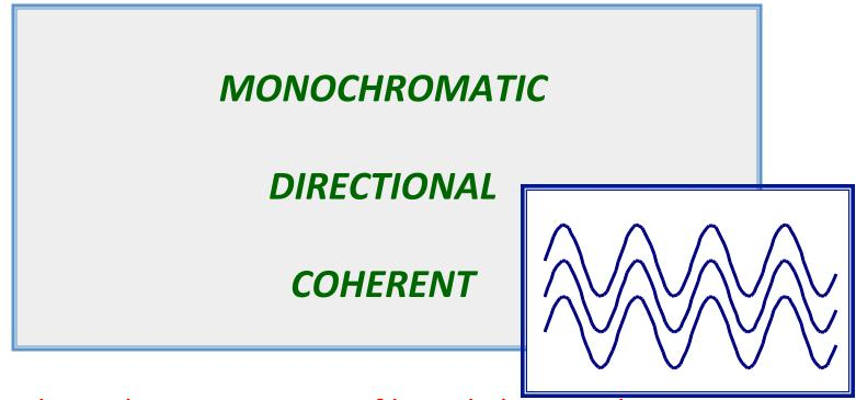
These three properties of laser light are what can make it more hazardous than ordinary light. Laser light can deposit a lot of energy within a small area.
